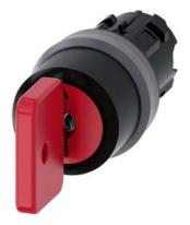
Key-operated switch O.M.R, 22 mm, round, plastic with metal front ring, lock number 73037, red, with 2 keys, 3 switch positions I-O-II, latching, actuating angle 2x45°, 10:30h/12h/13:30h, key removal O+I, with laser labeling, upper case and lower case, always upper case at the beginning of the word
