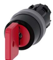
Key-operated switch O.M.R, 22 mm, round, plastic with metal front ring, lock number 73037, red, with 2 keys, 3 switch positions I-O-II, latching, actuating angle  $2x45^{\circ}$ , 10:30h/12h/13:30h, key removal O+I, with laser labeling, lower case
