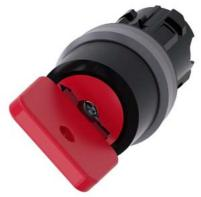
Key-operated switch O.M.R, 22 mm, round, plastic with metal front ring, lock number 73037, red, with 2 keys, 2 switch positions O-I, latching, actuating angle 90°, 10:30h/13:30h, key removal O+I, with laser labeling, lower case
