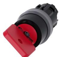
Key-operated switch O.M.R, 22 mm, round, plastic with metal front ring, lock number 73037, red, with 2 keys, 2 switch positions O-I, latching, actuating angle 90°, 10:30h/13:30h, key removal O+I, Z=50-unit packaging
