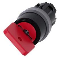
Key-operated switch O.M.R, 22 mm, round, plastic with metal front ring, lock number 73037, red, with 2 keys, 2 switch positions O-I, latching, actuating angle 90°, 10:30h/13:30h, key removal O, with laser labeling, inscription or symbol Customer-specific selection with SIRIUS ACT configurator (CIN)
