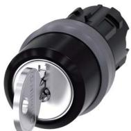
RONIS key-operated switch, 22 mm, round, plastic with metal front ring, lock number 455, with 2 keys, 3 switch positions I-O-II, latching, actuating angle 2x45°, 10:30h/12h/13:30h, key removal O, with laser labeling, inscription or symbol Customer-specific selection with SIRIUS ACT configurator (CIN)
