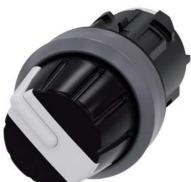
Selector switch, 22 mm, round, plastic with metal front ring, white, Rotary knob, 4 switch positions I-II-III-IV, latching, Actuating angle  $4x90^\circ$ , 3h/6h/9h/12h
