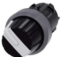
Selector switch, 22 mm, round, plastic with metal front ring, white, Rotary knob, 4 switch positions I-II-III-IV, latching, Actuating angle 4x90°, 3h/6h/9h/12h, with laser labeling, upper case and lower case, always upper case at the beginning of the word
