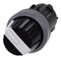
Selector switch, 22 mm, round, plastic with metal front ring, white, Rotary knob, 4 switch positions I-II-III-IV, latching, Actuating angle 4x90°, 3h/6h/9h/12h, with laser labeling, lower case
