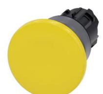
Mushroom pushbutton, 22 mm, round, plastic with metal front ring, yellow, 40mm, momentary contact type, with laser labeling, symbol number according to, ISO 7000 or IEC 60417
