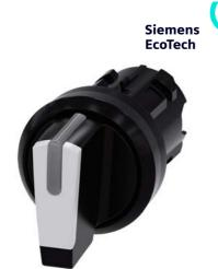
Selector switch, illuminable, 22 mm, round, plastic, white, selector switch, short, 3 switch positions I>O<II, momentary contact type, actuating angle  $2x45^{\circ}$ , 10:30h/12h/13:30h, with laser labeling, inscription or symbol Customer-specific selection with SIRIUS ACT configurator (CIN)
