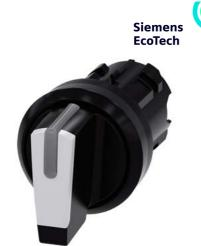
Selector switch, illuminable, 22 mm, round, plastic, white, selector switch, short, 3 switch positions I>O<II, momentary contact type, actuating angle 2x45°, 10:30h/12h/13:30h, with laser labeling, upper case and lower case, always upper case at beginning of line
