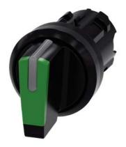
Selector switch, illuminable, 22 mm, round, plastic, green, selector switch, short, 3 switch positions I>O<II, momentary contact type, actuating angle 2x45°, 10:30h/12h/13:30h, with laser labeling, upper case and lower case, always upper case at beginning of line
