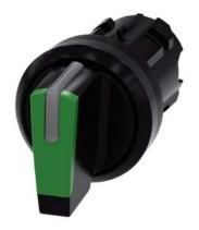
Selector switch, illuminable, 22 mm, round, plastic, green, selector switch, short, 3 switch positions I>O<II, momentary contact type, actuating angle  $2x45^{\circ}$ , 10:30h/12h/13:30h Z=50-unit packaging
