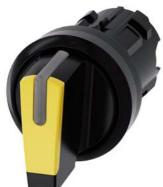
Selector switch, illuminable, 22 mm, round, plastic, yellow, selector switch, short, 3 switch positions |>O<I|, momentary contact type, actuating angle 2x45°, 10:30h/12h/13:30h, with laser labeling, upper case and lower case, always upper case at the beginning of the word
