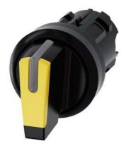
Selector switch, illuminable, 22 mm, round, plastic, yellow, selector switch, short, 3 switch positions I>O<II, momentary contact type, actuating angle  $2x45^{\circ}$ , 10:30h/12h/13:30h, with laser labeling, lower case
