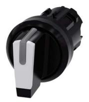
Selector switch, illuminable, 22 mm, round, plastic, white, selector switch, short, 3 switch positions I-O-II, latching, actuating angle 2x45°, 10:30h/12h/13:30h, with laser labeling, lower case
