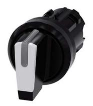
Selector switch, illuminable, 22 mm, round, plastic, white, selector switch, short, 3 switch positions I-O-II, latching, actuating angle 2x45°, 10:30h/12h/13:30h, with laser labeling, upper case
