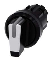
Selector switch, illuminable, 22 mm, round, plastic, white, selector switch, short, 3 switch positions I-O-II, latching, actuating angle 2x45°, 10:30h/12h/13:30h, with laser labeling, upper case and lower case, always upper case at beginning of line
