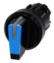
Selector switch, illuminable, 22 mm, round, plastic, blue, selector switch, short, 3 switch positions I-O-II, latching, actuating angle 2x45°, 10:30h/12h/13:30h, with laser labeling, upper case and lower case, always upper case at the beginning of the word
