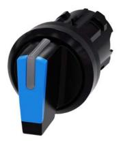
Selector switch, illuminable, 22 mm, round, plastic, blue, selector switch, short, 3 switch positions I-O-II, latching, actuating angle  $2x45^{\circ}$ , 10:30h/12h/13:30h, with laser labeling, upper case and lower case, always upper case at beginning of line
