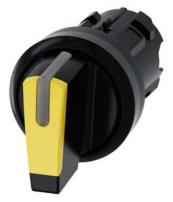
Selector switch, illuminable, 22 mm, round, plastic, yellow, selector switch, short, 3 switch positions I-O-II, latching, actuating angle 2x45°, 10:30h/12h/13:30h Z=50-unit packaging
