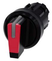
Selector switch, illuminable, 22 mm, round, plastic, red, selector switch, short, 3 switch positions I-O-II, latching, actuating angle 2x45°, 10:30h/12h/13:30h, with laser labeling, upper case and lower case, always upper case at the beginning of the word
