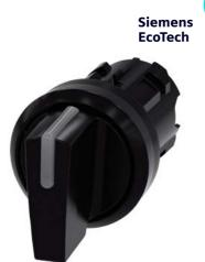
Illuminable selector switch, 22 mm, round, plastic, black, Selector switch short, 3 switch positions I-O-II, latching, actuating angle 2x45°, 10:30h/12h/13:30h
