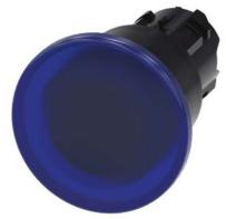
Illuminated mushroom pushbutton, 22 mm, round, plastic, blue, 40mm, latching, pull-to-unlatch mechanism, with laser labeling, upper case and lower case, always upper case at the beginning of the word
