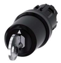
Key-operated switch IKON, 22 mm, round, plastic, special lock, with 2 keys, 3 switch positions I-O-II, latching, actuating angle 2x45°, 10:30h/12h/13:30h, Key removal I+O+II
