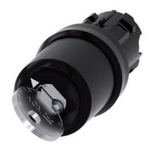
Key-operated switch IKON, 22 mm, round, plastic, lock number 360012K1, with 2 keys, 2 switch positions O-I, latching, actuating angle 90°, 10:30h/13:30h, key removal O+I, with laser labeling, upper case and lower case, always upper case at the beginning of the word
