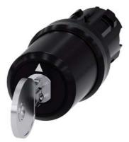
Key-operated switch BKS, 22 mm, round, plastic, Lock No. E9 (VW), without key, 3 switch positions I-O-II, latching, actuating angle  $2x45^{\circ}$ , 10:30h/12h/13:30h, Key removal I+O+II, with laser labeling, upper case
