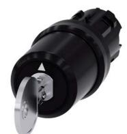
Key-operated switch BKS, 22 mm, round, plastic, Lock No. E9 (VW), without key, 3 switch positions I-O-II, latching, actuating angle 2x45°, 10:30h/12h/13:30h, Key removal I+O+II, with laser labeling, upper case and lower case, always upper case at beginning of line
