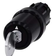
key-operated switch Siemens, 22 mm, round, plastic, lock number SSG10, with 2 keys, 3 switch positions I>O<II, momentary contact on the left, latching on the right, actuating angle 2x45°, 10:30h/12h/13:30h, key removal O+II
