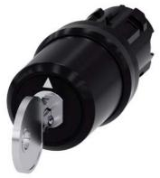
key-operated switch Siemens, 22 mm, round, plastic, lock number SSG10, with 2 keys, 3 switch positions I>O<II, momentary contact on the left, latching on the right, actuating angle  $2x45^{\circ}$ , 10:30h/12h/13:30h, key removal O
