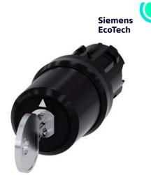
key-operated switch Siemens, 22 mm, round, plastic, lock number SSG10, with 2 keys, 3 switch positions I>O<II, momentary contact on the left, latching on the right, actuating angle 2x45°, 10:30h/12h/13:30h, key removal O, with laser labeling, inscription or symbol customer-specific selection with SIRIUS ACT configurator (CIN)
