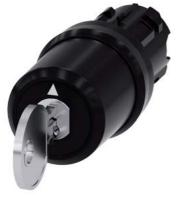
key-operated switch Siemens, 22 mm, round, plastic, lock number SSG10, with 2 keys, 3 switch positions I-O<II, left latching, momentary contact type on the right, actuating angle  $2x45^\circ$ , 10:30h/12h/13:30h, key removal O
