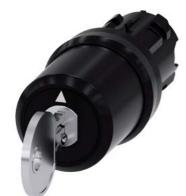
key-operated switch Siemens, 22 mm, round, plastic, lock number SSG10, with 2 keys, 3 switch positions I-O-II, latching, actuating angle 2x45°, 10:30h/12h/13:30h, key removal I+II
