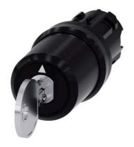
key-operated switch Siemens, 22 mm, round, plastic, lock number SSG10, with 2 keys, 3 switch positions I-O-II, latching, actuating angle 2x45°, 10:30h/12h/13:30h, key removal I+O+II, with laser labeling, upper case and lower case, always upper case at beginning of line
