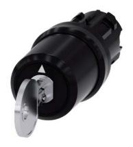
key-operated switch Siemens, 22 mm, round, plastic, lock number SSG10, with 2 keys, 3 switch positions I-O-II, latching, actuating angle 2x45°, 10:30h/12h/13:30h, key removal O, with laser labeling, upper case and lower case, always upper case at the beginning of the word
