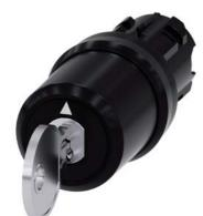
key-operated switch Siemens, 22 mm, round, plastic, lock number SSG10, with 2 keys, 3 switch positions I-O-II, latching, actuating angle 2x45°, 10:30h/12h/13:30h, key removal O Z=50-unit packaging
