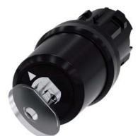
key-operated switch Siemens, 22 mm, round, plastic, lock number SSG10, with 2 keys, 2 switch positions O-I, latching, actuating angle 90°, 10:30h/13:30h, key removal O+I, with laser labeling, upper case and lower case, always upper case at the beginning of the word
