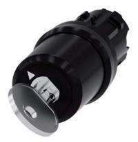
key-operated switch Siemens, 22 mm, round, plastic, lock number SSG10, with 2 keys, 2 switch positions O-I, latching, actuating angle 90°, 10:30h/13:30h, key removal O+I, with laser labeling, lower case
