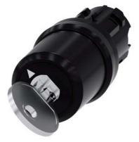
key-operated switch Siemens, 22 mm, round, plastic, lock number SSG10, with 2 keys, 2 switch positions O-I, latching, actuating angle 90°, 10:30h/13:30h, key removal O+I Z=50-unit packaging
