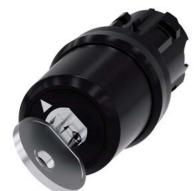
key-operated switch Siemens, 22 mm, round, plastic, lock number SSG10, with 2 keys, 2 switch positions O-I, latching, actuating angle 90°, 10:30h/13:30h, key removal O
