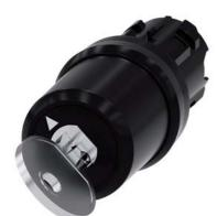
key-operated switch Siemens, 22 mm, round, plastic, special lock, with 2 keys, 2 switch positions O-I, latching, actuating angle  $90^\circ$ , 10:30h/13:30h, key removal O
