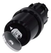
key-operated switch Siemens, 22 mm, round, plastic, lock number SSG10, with 2 keys, 2 switch positions O-I, latching, actuating angle 90°, 10:30h/13:30h, key removal O Z=50-unit packaging
