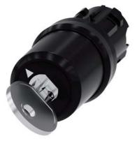
key-operated switch Siemens, 22 mm, round, plastic, lock number SSG10, with 2 keys, 2 switch positions O<I, momentary contact type, actuating angle 45°, 10:30h/12h, key removal O, with laser labeling, inscription or symbol customer-specific selection with SIRIUS ACT configurator (CIN)
