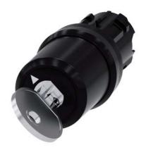
key-operated switch Siemens, 22 mm, round, plastic, lock number SSG10, with 2 keys, 2 switch positions O<I, momentary contact type, actuating angle  $45^\circ,$  10:30h/12h, key removal O, with laser labeling, upper case
