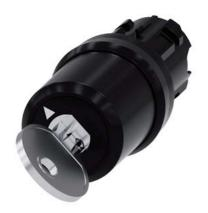
key-operated switch Siemens, 22 mm, round, plastic, special lock, with 2 keys, 2 switch positions O<I, momentary contact type, actuating angle 45°, 10:30h/12h, key removal O
