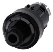
ID key-operated switch, 22 mm, round, plastic, black, RFID, 4 switch positions O-II-III, operating angle 3x45°, without ID key, Key removal in O+I+II+III, Z=50-unit packaging
