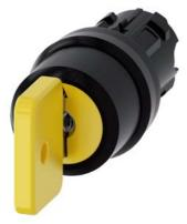
Key-operated switch O.M.R, 22 mm, round, plastic, lock number 73033, yellow, with 2 keys, 3 switch positions I-O-II, latching, actuating angle 2x45°, 10:30h/12h/13:30h, Key removal I+O+II, with laser labeling, upper case
