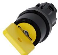
Key-operated switch O.M.R, 22 mm, round, plastic, lock number 73033, yellow, with 2 keys, 2 switch positions O-I, latching, actuating angle 90°, 10:30h/13:30h, key removal O+I, with laser labeling, upper case and lower case, always upper case at the beginning of the word
