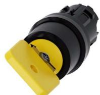
Key-operated switch O.M.R, 22 mm, round, plastic, lock number 73033, yellow, with 2 keys, 2 switch positions O<I, momentary contact type, Actuating angle 45°, 10:30h/12h, Key removal O
